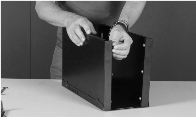
Mount the back plate 4 . First turn bolts (6x) in the sidewall, do not tighten. Then slide the back plate in and tighten the bolts (6x).
