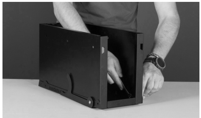
Mount the front legs 6 (2x bolt + 2x lock nuts). Do not tighten the lock nuts too tight, the legs have to be able to move.
